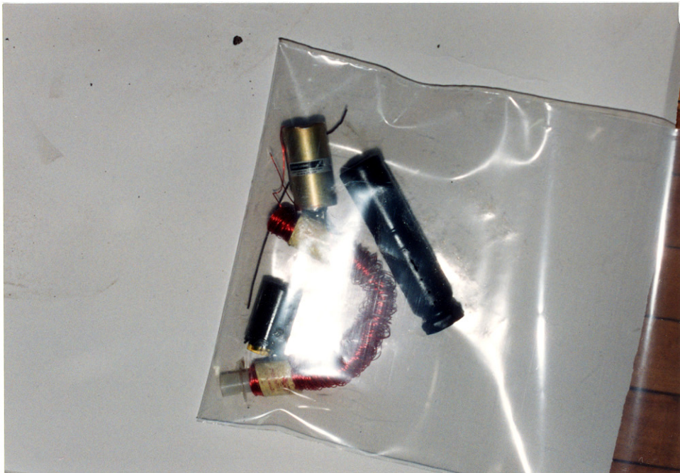
52. View of internal valve components of the failed CNG tank
